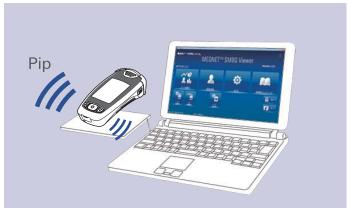
Transfers data wirelessly using RFID.
